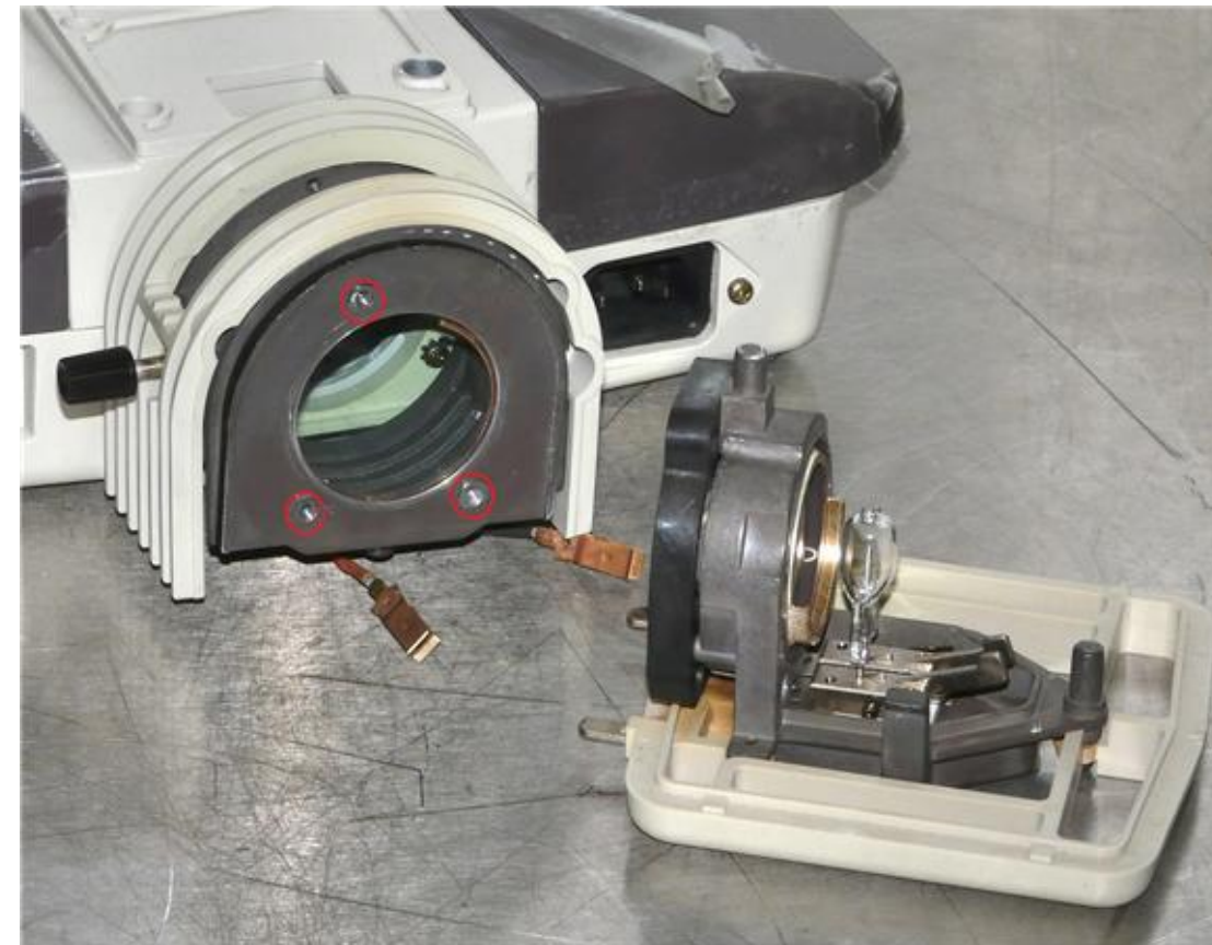
(4) Remove Lamp housing from microscope.
