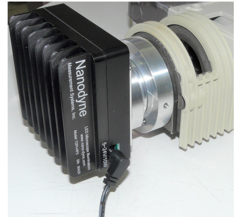
(6) Connect the power supply and the new illuminator is ready to operate.
