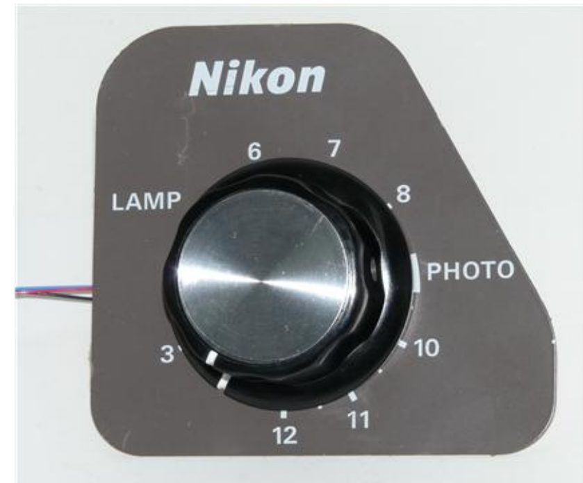
(4) Attach the new knob provided, using a small flat blade screwdriver
