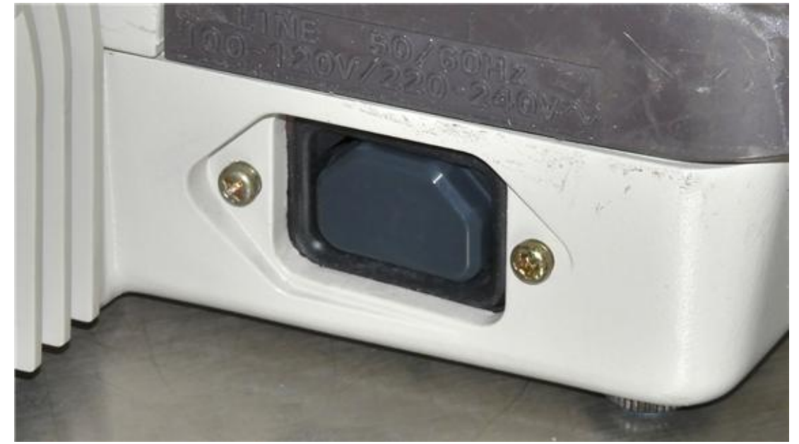
(4) Silicone rubber blocking plug installed in AC power receptacle.
