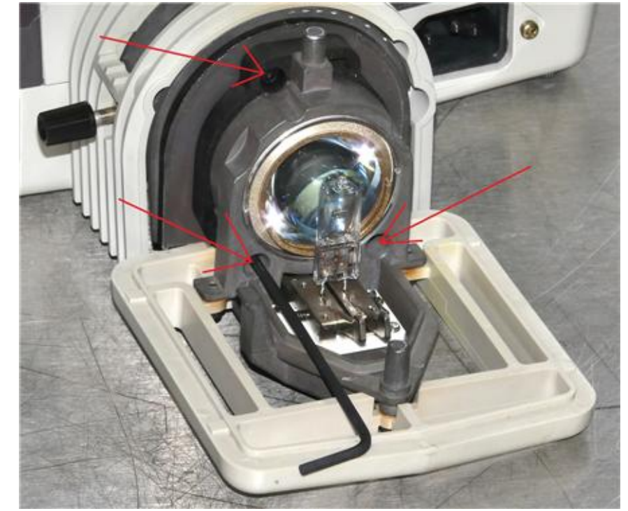
(3) Remove the 3 screws holding the lamp housing to the microscope with the 2.5mm hex key provided.
