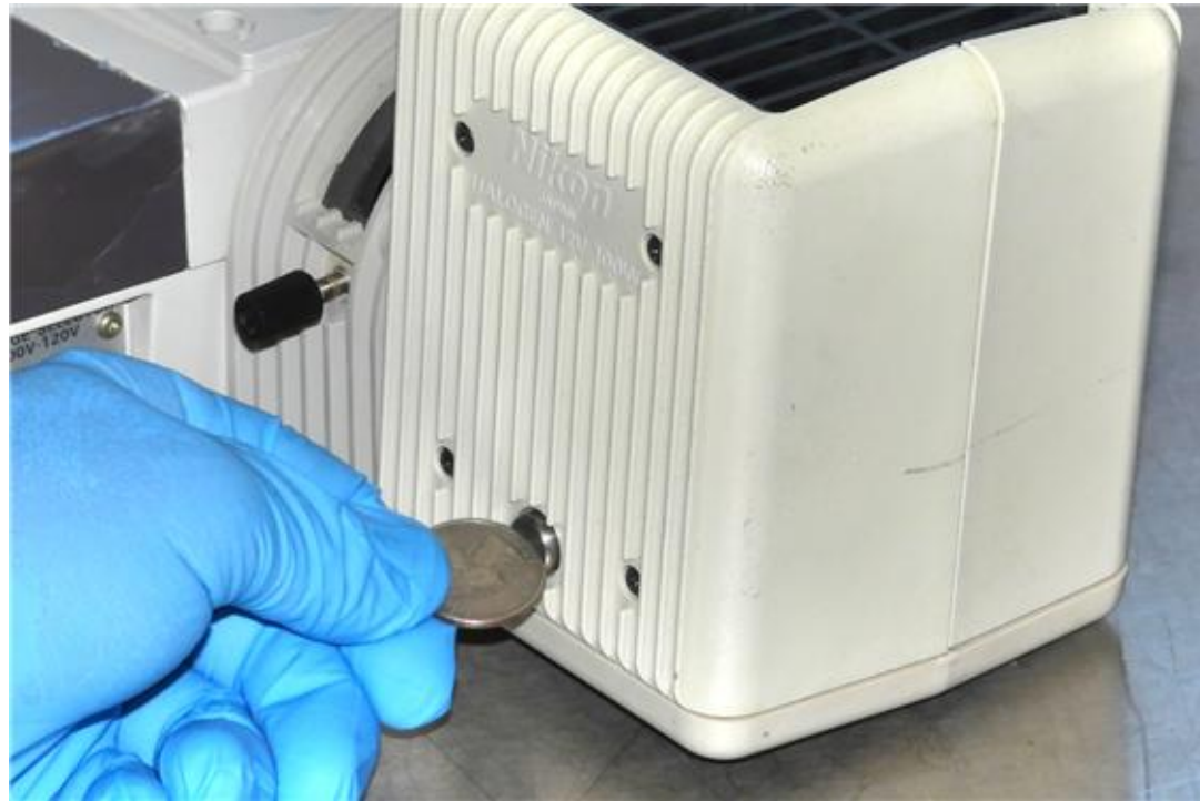
(1) Loosen the screw holding the lamp cover.
