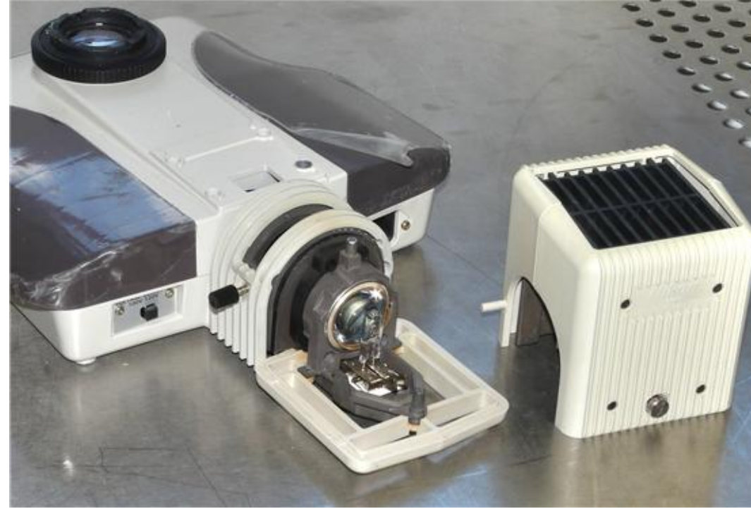
(2) Lift the cover off the lamp housing.
